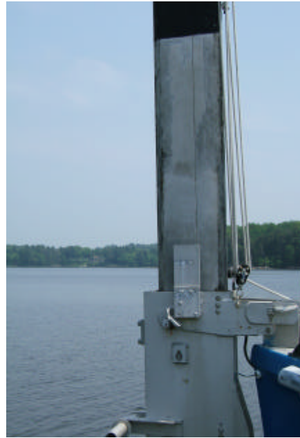
Figure 5: Pole mounting in the RV Coastal Surveyor bow
