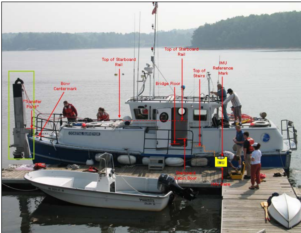
Figure 2. General overview of IMU to Bow Centermark measurement locations.
