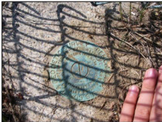
Figure 2 - Left photo is a close up of benchmark NO 1 1919. Right photo is looking NE with benchmark NO 1 1919 in the foreground. Note the NOAA tide gauge (Station number 8423898) at the SW corner of the covered dock.
