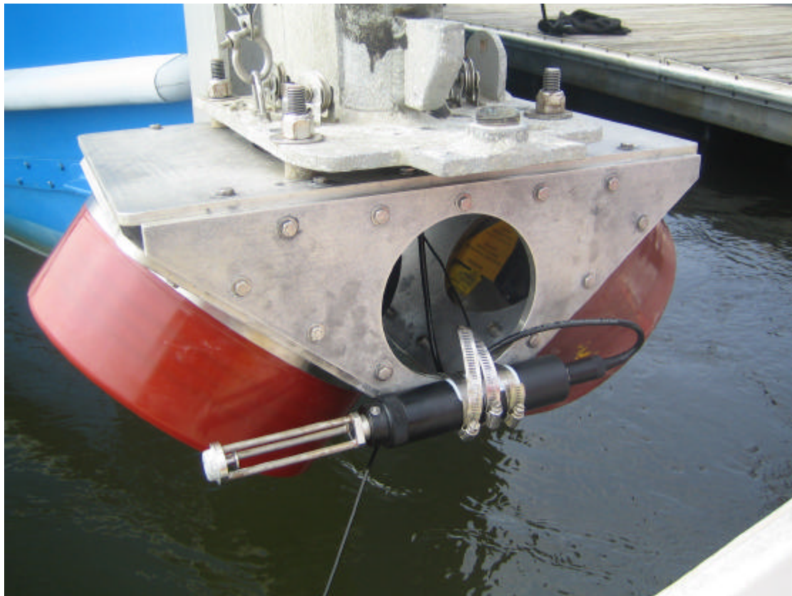
Figure 3: Smart SV&T Surface Sound Speed unit mounted with Transducers
