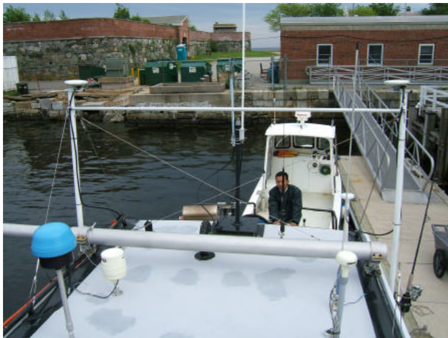
Figure 6: POS/MV antennas mounted on the R/V Coastal Surveyor (top-rear view)
