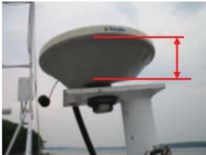
Figure 2: Vendor provided Phase offset from base of Antenna
