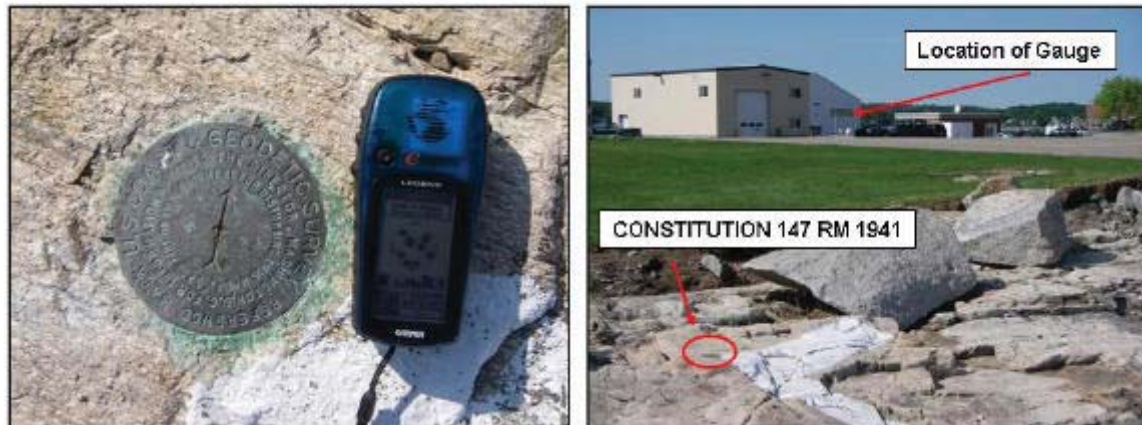
Figure 6 – Left photo is a close up of benchmark CONSTITUTION 147 NO 1 1941. Right photo is looking NNE from benchmark CONSTITUTION 147 NO 1941 and shows the location of the backup tide gauge in the background.
