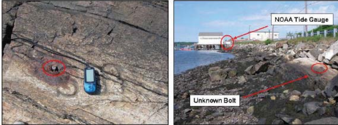
Figure 3 - Left photo shows BM 4 which is an iron bolt drilled into a bedrock out crop. Right photo is looking NE and shows the NOAA tide gauge in the background.
