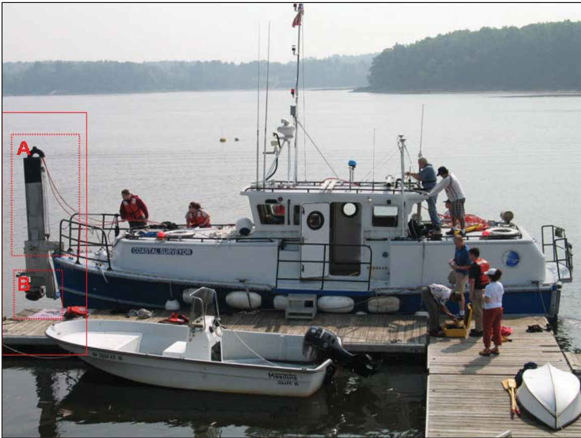
Figure 3. General overview of Bow Centermark to Port and Starboard Transducer offset measurement locations (see insets A and B).
