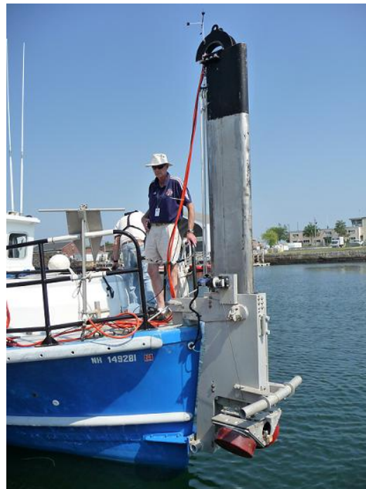
Figure 6: EM 3002 transducers bow-mounted on the R/V Coastal Surveyor
