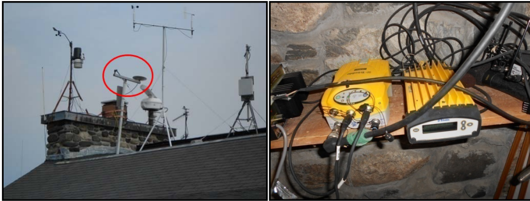
Figure 4. RTK GPS base station at the Seacoast Science Center at Odiorne State Park, NH, includes the radio and GPS antennas (left), and Trimble radio modem and GPS receiver (right)
