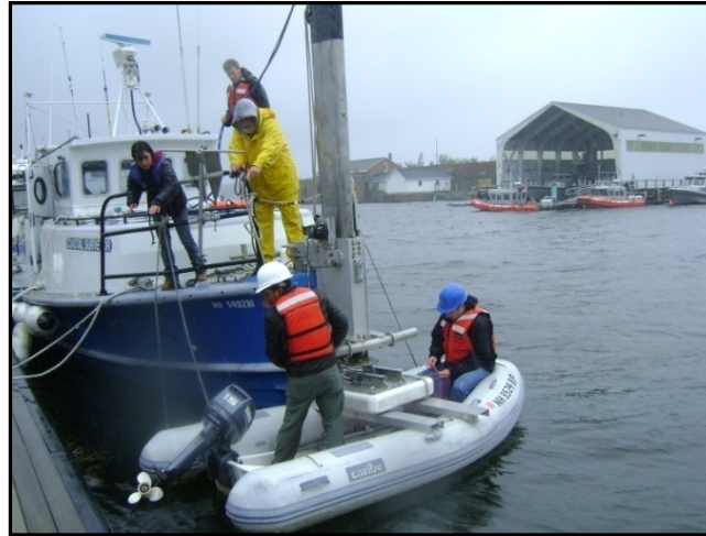
Figure 7. Installation of the Kongsberg EM2040 on the bow ram of the R/V Coastal Surveyor
