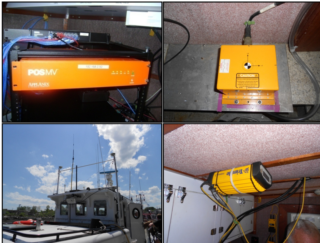
Figure 3. Components of the POS M/V 320 v4 integration on the R/V Coastal Surveyor include the POS computer system (top left), IMU (top right), GPS antennas (bottom left), and RTK receiver (bottom right)
