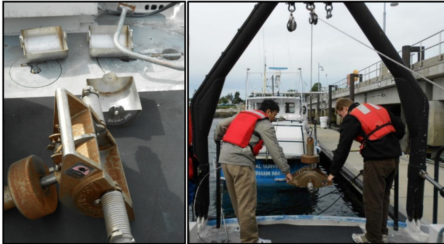
Figure 6. Wildco Shipek grab sampler, on deck (left), and lowered by cable winch on the A-frame of R/V Cochecho
