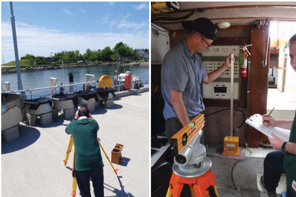
Figure 2. A self leveling surveyor's level was used to measure the vertical offset from the IMU to Antenna. Inside the cabin, a laser was set on top of the level as the distance was too short to focus the telescope.
