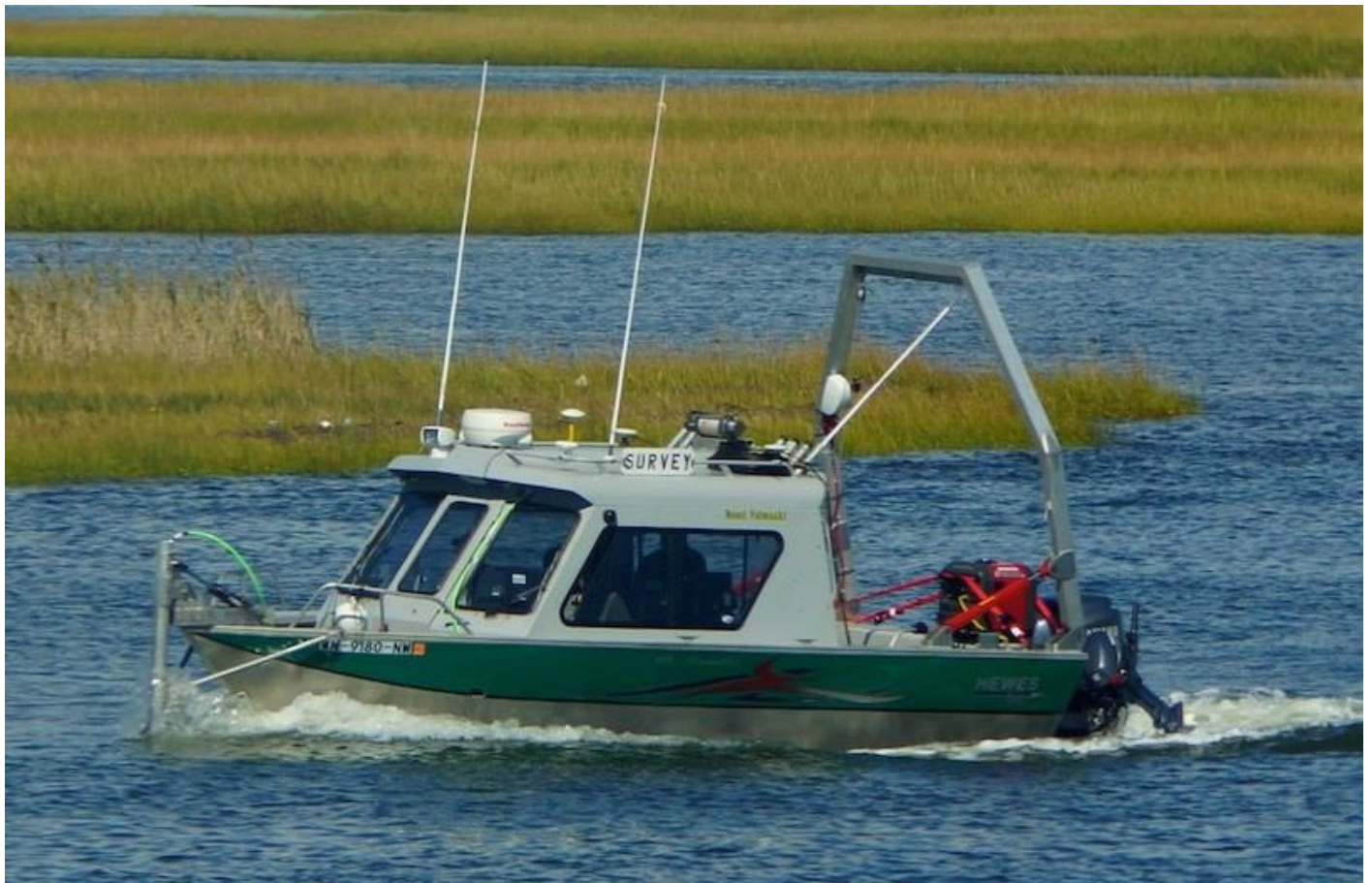
Figure 5: M/V Nooit Volmaakt from the port side. The pole mount on the bow for the Edge Tech SSS can be seen.
