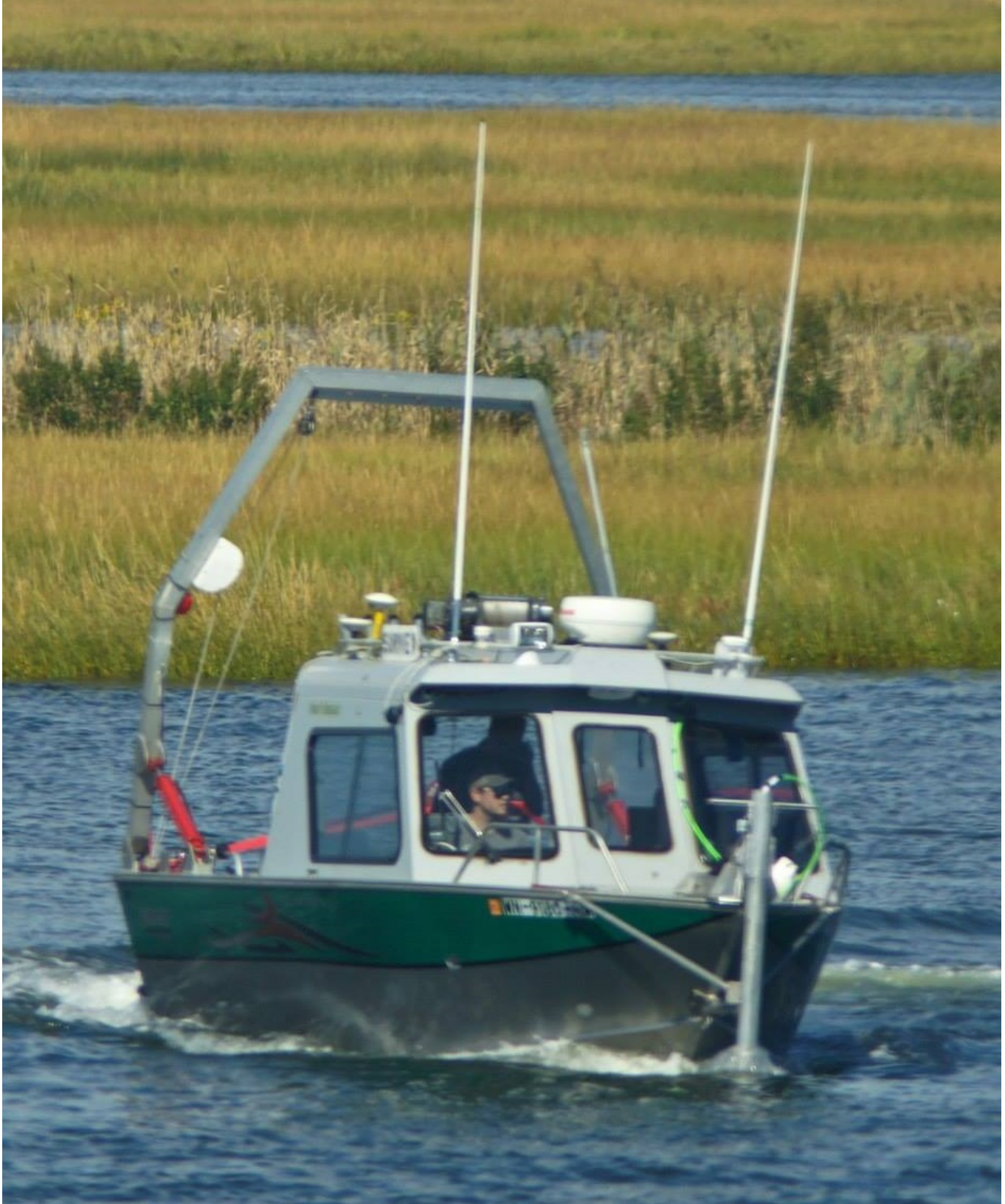
Figure 6: M/V Nooit Volmaakt from the starboard bow. The pole mount on the bow for the Edge Tech SSS can be seen.
