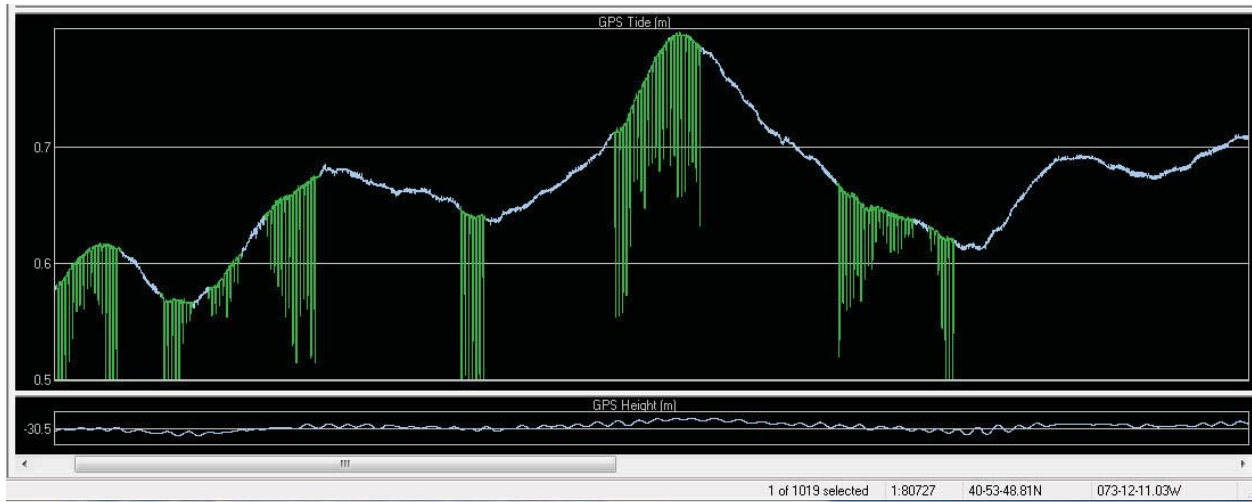
Figure 11: Altitude Anomaly as viewed in Attitude Editor (GPS Tide). The green is displaying unusual GPS Tide levels.
