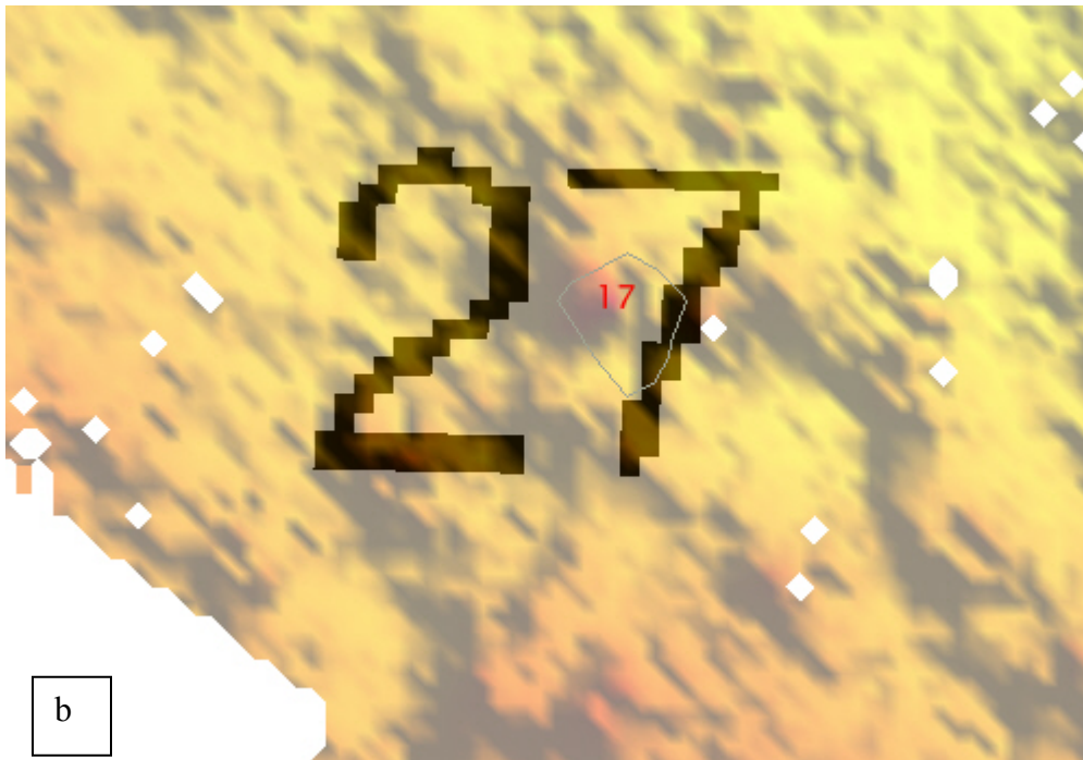
Rock with least depth of 17ft, located at latitude 42-15-53.99N, longitude 070-45-45.43W (a). Chart 13269, edition 10, 20060201; the current sounding is at 27ft, the new sounding is depicted in red (b).
