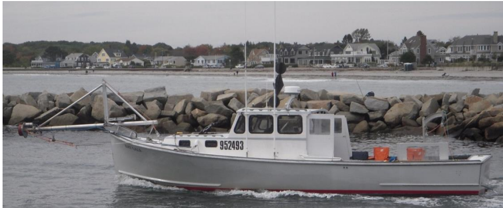
Figure 3. Survey vessel F/V Amy Gale shown with pole-mounted hardware in raised position during transit.
