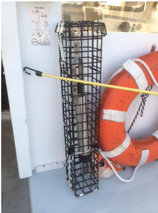
Figure 4: Digibar S in its protective cage.
