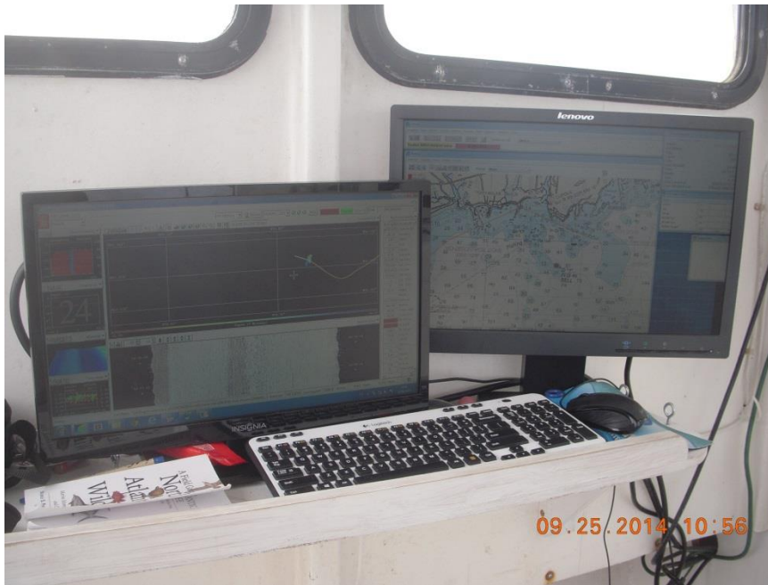
Figure 8: Work station with SIS display on right and Hypack on left.
