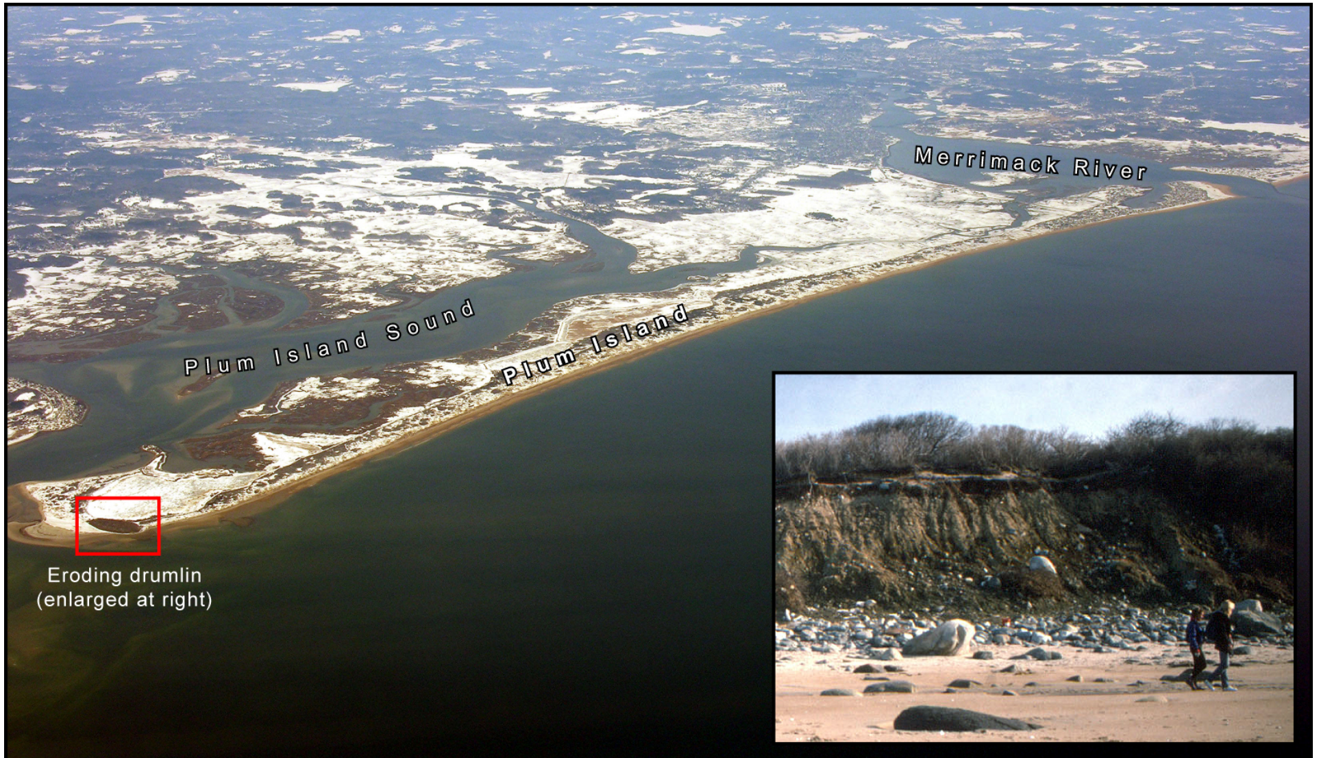
Figure 1.3. Air photograph of Plum Island and the mouth of the Merrimack River on the northeastern coast of Massachusetts. A small drumlin (inset) anchors the southern end of the island. Erosion of the drumlin provides sandy sediment to the barrier beach and has left behind a deposit of boulders on the beach and shoreface. (Photograph by Joseph Kelley, University of Maine, March 2005.)
