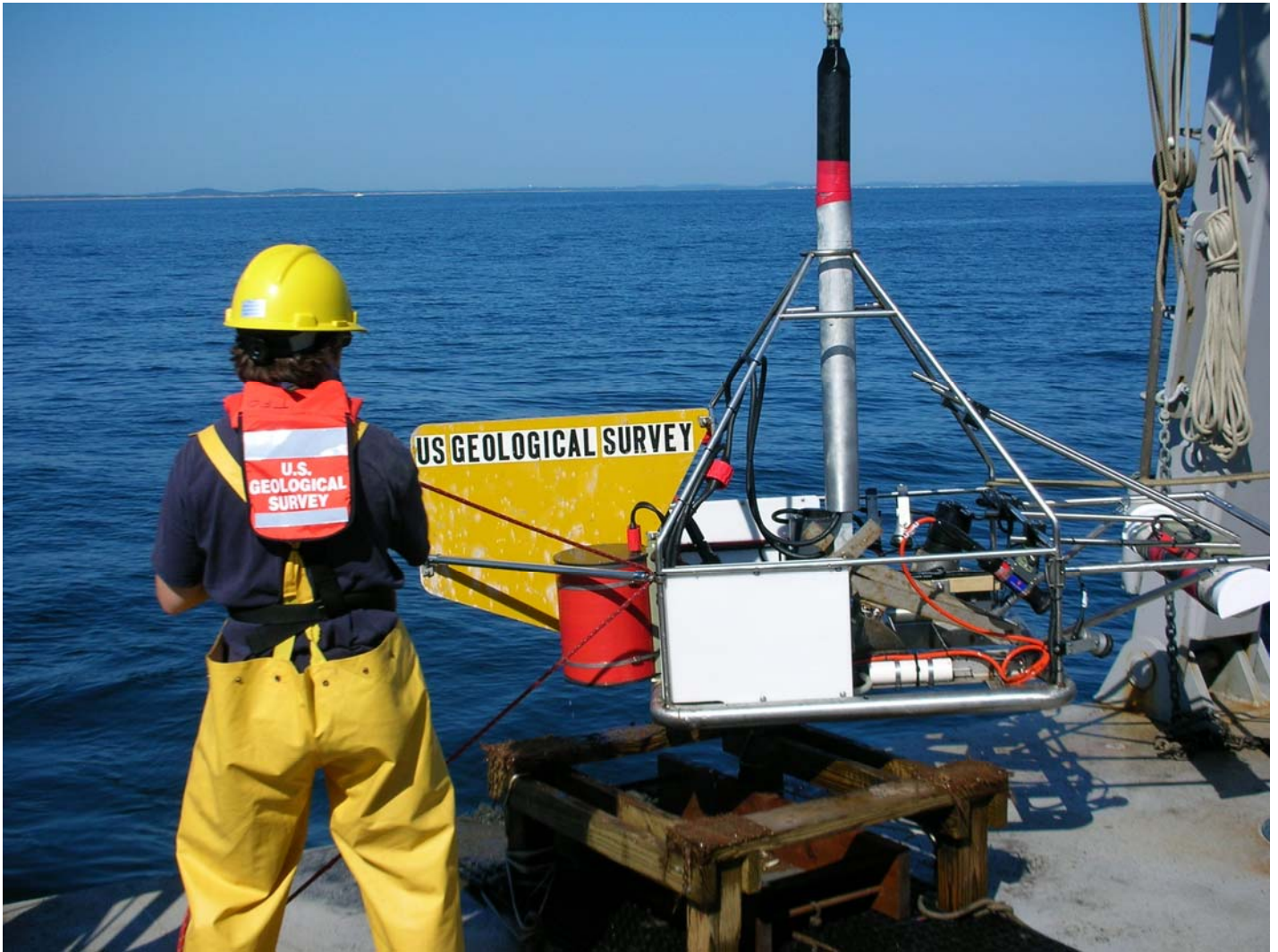
Figure 3.8. Photograph of the SEABed Observation and Sampling System (SEABOSS) on the deck of the RV Connecticut . Photographic data and sediment samples collected by the system were used to validate geophysical data and characterize seafloor environments.
